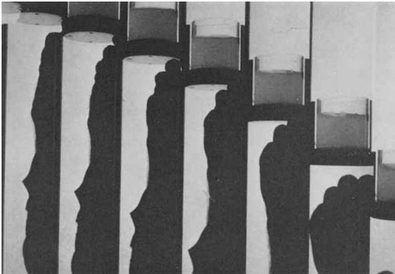
FIGURE 7. A sequence of photographs of the vessel containing soap solution taken 0.033 sec apart just as the vessel is released from rest. Note the motion of the free surface during free fall.
